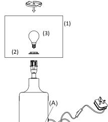
To use this item in Europe, the 3 pin adaptor can be removed by loosening the central screw and removing the adaptor to reveal the 2 pin Europe plug.
